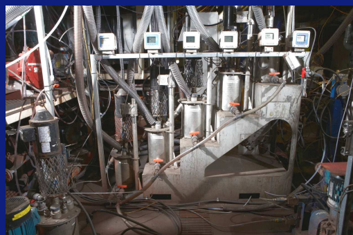
Leach Skid: 4-stage atmospheric leach in either 316 SS or Ti-2 tanks (~15 Liters)
