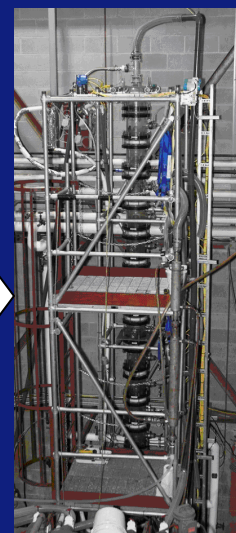
Distillation column: 15 stages – Max. feed ~180 kg/hr of liquid
