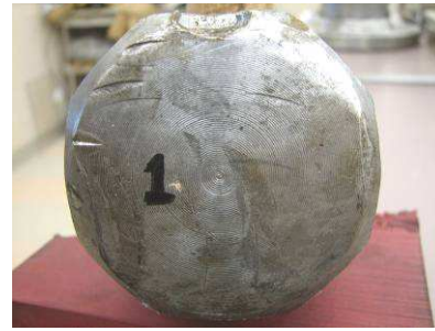
Above: The face of the hammer that chipped.
