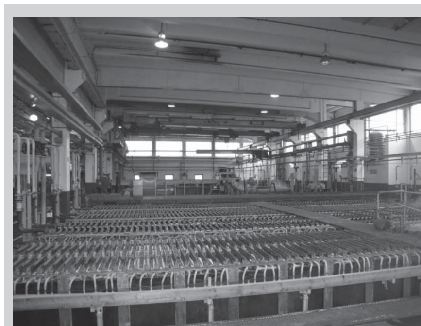
Figure 5. Cobalt electrowinning cell house at Xstrata Nikkelverk AS.
